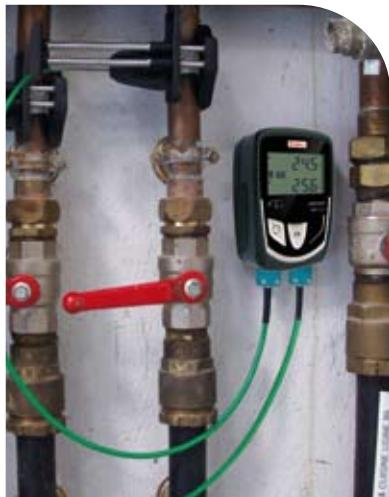
With **Velcro probes** or **spring clamp probes**, KTT 310 is a key instrument to control and monitor your **hot water / sanitary network**.
